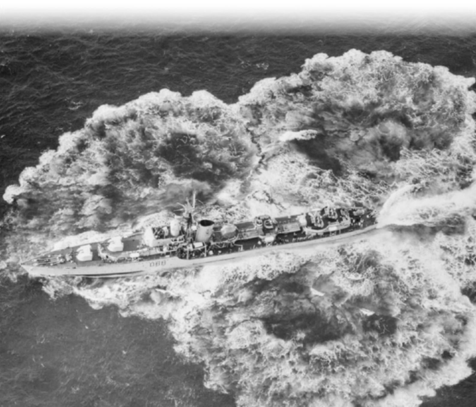
HMS Barrosa in a post-war exercise, steaming through the pattern which the exploding charges from her Squid Anti Submarine weapon firing its missiles ahead of the ship had made a few seconds earlier. See 31 July. Image from the Imperial War Museum collection (© IWM (A 33111))
